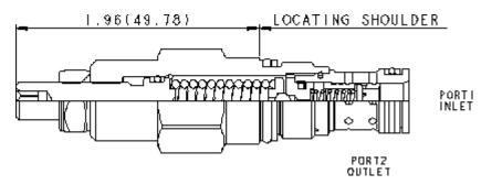
Kick-down relief cartridges act similar to a circuit breaker in an electrical system. The valves will kick completely open and remain open once the pressure at the inlet (port 1) exceeds the valve setting, creating an unrestricted flow path from port 1 to tank (port 2). The valve remains open as long as the pressure at port 1 exceeds the pressure at port 2. To reset the valve, flow from port 1 to port 2 must cease and pressure at port 2 must be equal to or greater than the pressure at port 1.
