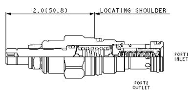
Kick-down relief cartridges act similar to a circuit breaker in an electrical system. The valves will kick completely open and remain open once the pressure at the inlet (port 1) exceeds the valve settting, creating an unrestricted flow path from port 1 to tank (port 2). The valve remains open as long
