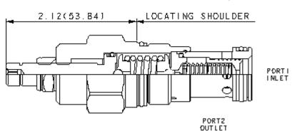
Kick-down relief cartridges act similar to a circuit breaker in an electrical system. The valves will kick completely open and remain open once the pressure at the inlet (port 1) exceeds the valve setting, creating an unrestricted flow path from port 1 to tank (port 2). The valve remains open as long as the pressure at port 1 exceeds the pressure at port 2. To reset the valve, flow from port 1 to port 2 must cease and pressure at port 2 must be equal to or greater than the pressure at port 1.
