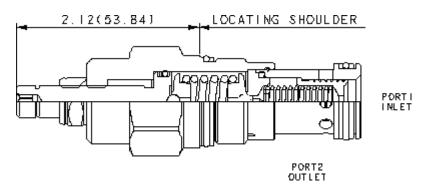
Kick-down relief cartridges act similar to a circuit breaker in an electrical system. The valves will kick completely open and remain open once the pressure at the inlet (port 1) exceeds the valve settling, creating an unrestricted flow path from port 1 to tank (port 2). The valve remains open as long
