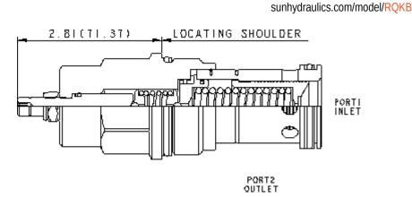
Kick-down relief cartridges act similar to a circuit breaker in an electrical system. The valves will kick completely open and remain open once the pressure at the inlet (port 1) exceeds the valve setting, creating an unrestricted flow path from port 1 to tank (port 2). The valve remains open as long as the pressure at port 1 exceeds the pressure at port 2. To reset the valve, flow from port 1 to port 2 must cease and pressure at port 2 must be equal to or greater than the pressure at port 1.
