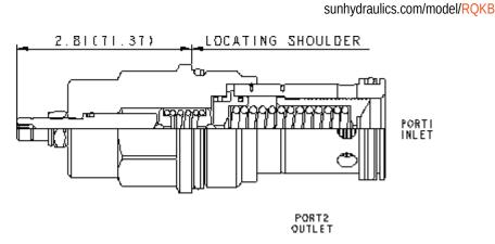
Kick-down relief cartridges act similar to a circuit breaker in an electrical system. The valves will kick completely open and remain open once the pressure at the inlet (port 1) exceeds the valve setting, creating an unrestricted flow path from port 1 to tank (port 2). The valve remains open as long as the pressure at port 1 exceeds the pressure at port 2. To reset the valve, flow from port 1 to port 2 must cease and pressure at port 2 must be equal to or greater than the pressure at port 1.
