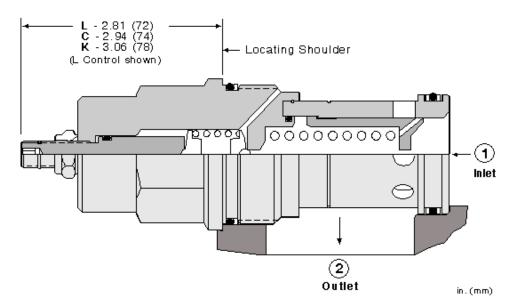
Kick-down relief cartridges act similar to a circuit breaker in an electrical system. The valves will kick completely open and remain open once the pressure at the inlet (port 1) exceeds the valve setting, creating an unrestricted flow path from port 1 to tank (port 2). The valve remains open as long as the pressure at port 1 exceeds the pressure at port 2. To reset the valve, flow from port 1 to port 2 must cease and pressure at port 2 must be equal to or greater than the pressure at port 1.
