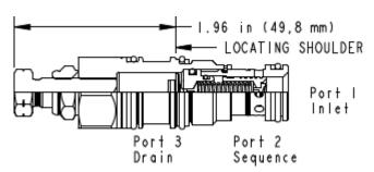
Pilot-operated, balanced piston sequence valves will supply a secondary circuit with flow once the pressure at the inlet (port 1) has exceeded the valve setting. The pressure setting of a sequence valve controls the pressure at port 1 relative to the pressure at the drain (port 3). These valves are insensitive to back pressure at port 2 (sequence), up to the valve setting. They may be used to regulate pressure in place of 2-port relief valves if there is pressure in the return line.
