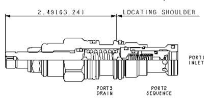
Pilot-operated, balanced poppet sequence valves will supply a secondary circuit with flow once the pressure at the inlet (port 1) has exceeded the valve setting. The pressure setting of a sequence valve controls the pressure at port 1 relative to the pressure at the drain (port 3). These valves are insensitive to back pressure at port 2 (sequence), up to the valve setting. They may be used to regulate pressure in place of 2-port relief valves if there is pressure in the return line.
