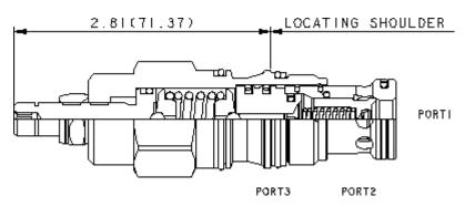
Pilot-operated, balanced poppet sequence valves will supply a secondary circuit with flow once the pressure at the inlet (port 1) has exceeded the valve setting. The pressure setting of a sequence valve controls the pressure at port 1 relative to the pressure at the drain (port 3). These valves are insensitive to back pressure at port 2 (sequence), up to the valve setting. They may be used to regulate pressure in place of 2-port relief valves if there is pressure in the return line.
