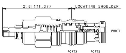
Pilot-operated, balanced poppet sequence valves will supply a secondary circuit with flow once the pressure at the inlet (port 1) has exceeded the valve setting. The pressure setting of a sequence valve controls the pressure at port 1 relative to the pressure at the drain (port 3). These valves are insensitive to back pressure at port 2 (sequence), up to the valve setting. They may be used to regulate pressure in
