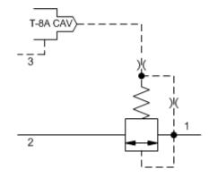
VALVE REQUIRED FOR PILOT CONTROL MUST BE ORDERED SEPARATELY. MODEL RBAP-\*\*\* PROPORTIONAL RELIEF SHOWN. 3.33 (84,7) MAXIMUM 2.31 (58,7) LOCATING SHOULDER EО INLET  $\overline{a}$  $\overline{\mathbf{n}}$ lĥ (1)(3) (2)DRAIN SEQUENCE in. (mm)
