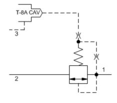
Valve required for pilot control must be ordered separately. Model RBAP-\*\*\* proportional relief shown. 3.33 (84,7) MAXIMUM Locating Shoulder 2.31 (58,7) π'' Ъп INLET D.Ém (1) 3 (2)Coil for Model RBAP-\*\*\* must be ordered separately DRAIN SEQUENCE
