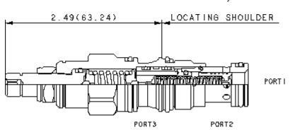
Three-port normally closed modulating elements with relief provide two functions when combined with an external orifice. The mainstage is a bypass compensator that controls a priority flow into the circuit, determined by the external orifice. Input flow in excess of the priority flow is bypassed to tank (port 2). If the inlet (port 1) pressure rises to the valve setting, the valve operates as a normal relief valve.
