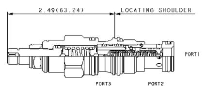
Three-port normally closed modulating elements with relief provide two functions when combined with an external orifice. The mainstage is a bypass compensator that controls a priority flow into the circuit, determined by the external orifice. Input flow in excess of the priority flow is bypassed to tank (port 2). If the inlet (port 1) pressure rises to the valve setting, the valve operates as a normal relief valve.
