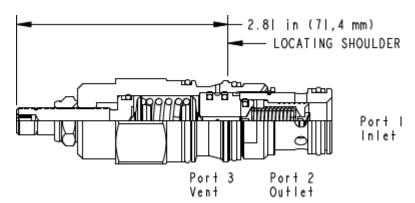
Ventable, pilot-operated, balanced piston relief cartridges are normally closed pressure regulating valves. When the pressure at the inlet (port 1) reaches the valve setting, the valve starts to open to tank (port 2), throttling flow to regulate the pressure. They provide a vent port (port 3) that connects between the main piston and pilot stage to provide for remote control by other pilot or 2-way valves. These valves
