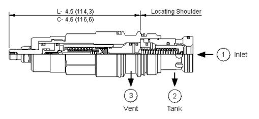
Ventable, pilot-operated, anti shock relief cartridges limit maximum system pressure and also limit the rate of pressure rise. The valve opens and then ramps closed at a constant speed, independent of settings and flows. These 3 port valves include a vent port (port 3) that connects between the main piston and the pilot stage to provide for remote control by other pilot or 2-way valves. The adjust screw determines the maximum (relief) setting and the minimum (threshold) setting.
