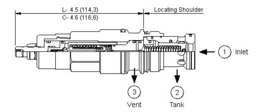
Ventable, pilot-operated, anti shock relief cartridges limit maximum system pressure and also limit the rate of pressure rise. The valve opens and then ramps closed at a constant speed, independent of settings and flows. These 3 port valves include a vent port (port 3) that connects between the main piston and the pilot stage to provide for remote control by other pilot or 2-way valves. The adjust screw determines the maximum (relief) setting and the minimum (threshold) setting.
