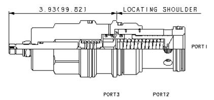
Three-port normally closed modulating elements with relief provide two functions when combined with an external orifice. The mainstage is a bypass compensator that controls a priority flow into the circuit, determined by the external orifice. Input flow in excess of the priority flow is bypassed to tank (port 2). If the inlet (port 1) pressure rises to the valve setting, the valve operates as a normal relief valve.
