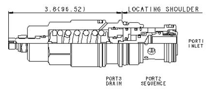
Direct-acting sequence valves with reverse-flow check will supply a secondary circuit with flow once the pressure at the inlet (port 1) has exceeded the valve setting. Additionally, these valves incorporate an integral check valve to provide reverse flow from port 2 (sequence) to port 1 (inlet). The pressure setting of a sequence valve controls the pressure at port 1 relative to the pressure at the drain (port 3).
