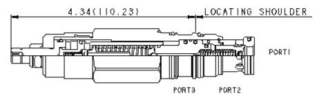
Pilot-operated, anti shock sequence cartridges limit maximum system pressure and also limit the rate of pressure rise. The valve opens and then ramps closed at a constant speed, independent of settings and flows. The adjust screw determines the maximum (relief) setting and the minimum (threshold) setting. The external drain makes the valve insensitive to pressure at port 2.
