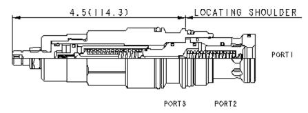
Pilot-operated, anti shock relief cartridges limit maximum system pressure and also limit the rate of pressure rise. The valve opens and then ramps closed at a constant speed, independent of settings and flows. The adjust screw determines the maximum (relief) setting and the minimum (threshold) setting. The external drain makes the valve insensitive to pressure at port 2.
