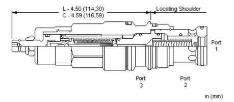
Pilot-operated, anti shock relief cartridges limit maximum system pressure and also limit the rate of pressure rise. The valve opens and then ramps closed at a constant speed, independent of settings and flows. The adjust screw determines the maximum (relief) setting and the minimum (threshold) setting. The external drain makes the valve insensitive to pressure at port 2.
