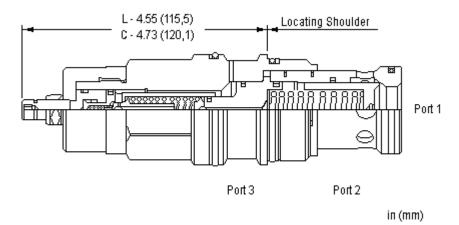
Pilot-operated, anti shock sequence cartridges limit maximum system pressure and also limit the rate of pressure rise. The valve opens and then ramps closed at a constant speed, independent of settings and flows. The adjust screw determines the maximum (relief) setting and the minimum (threshold) setting. The external drain makes the valve insensitive to pressure at port 2.
