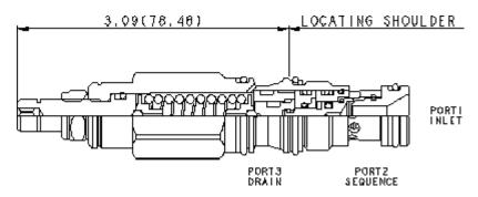
Direct-acting sequence valves will supply a secondary circuit with flow once the pressure at the inlet (port 1) has exceeded the valve setting. The pressure setting of a sequence valve controls the pressure at port 1 relative to the pressure at the drain (port 3).
