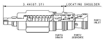
Direct-acting sequence valves will supply a secondary circuit with flow once the pressure at the inlet (port 1) has exceeded the valve setting. The pressure setting of a sequence valve controls the pressure at port 1 relative to the pressure at the drain (port 3).
