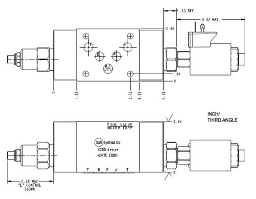
This assembly consists of a fully-adjustable, pressure-compensated flow control with reverse-flow check which provides precise flow regulation for meter-in or meter-out applications where there may be wide pressure fluctuations. It is infinitely adjustable from nearly closed up to the maximum flow. An integral high-capacity check valve provides unrestricted flow in the reverse direction. The rapid or feed rate is selected by a solenoid operated (normally open or closed) 2-way, 2-position valve.
