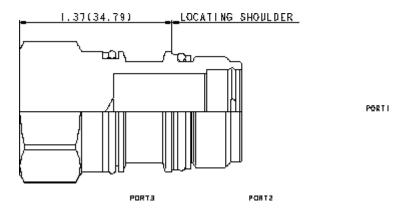
This cavity plug allows ports 1 and 2 to remain open and blocks port 3.
