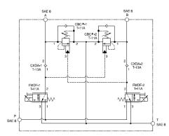
sunhydraulics.com/model/XCCL This valve assembly provides independent, proportional meter-in speed control for ports A and B, overrunning load control, and load-port relief protection. It also supplies makeup oil and flushes hot dirty oil out of the actuator. All oil coming out of the actuator returns to tank through port T.
