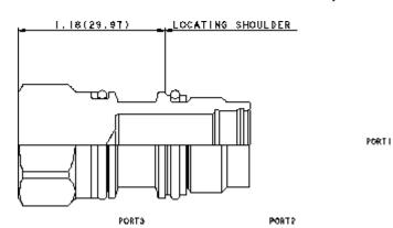
This cavity plug allows ports 1 and 2 to remain open and blocks port 3.
