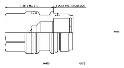
This cavity plug allows ports 1 and 2 to remain open and blocks port 3.
