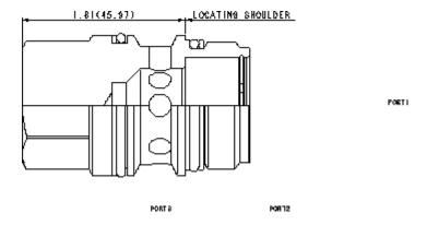
This cavity plug allows all ports to remain open.
