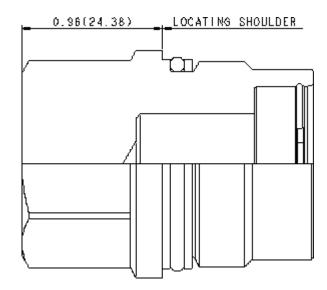
These cavity plugs can be used for both two-port and four-port cavities and allow all ports to remain connected.
