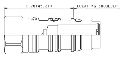
These cavity plugs can be used for both four-port and six-port cavities. When used in four-port cavities (T-21A, T-22A, T-23A and T-24A), ports 1 and 2 remain connected and ports 3 and 4 are blocked. When used in six-port cavities (T-61A, T-62A, T-63A and T-64A), ports 1, 2, 3 and 4 remain connected and ports 5 and 6 are blocked.
