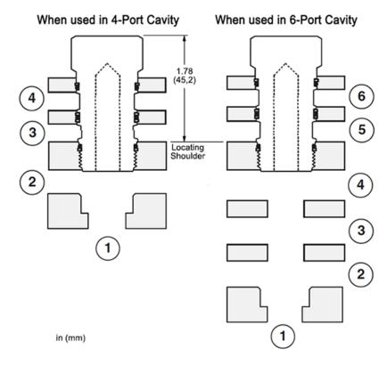
These cavity plugs can be used for both four-port and six-port cavities. When used in four-port cavities (T-21A, T-22A, T-23A and T-24A), ports 1 and 2 remain connected and ports 3 and 4 are blocked. When used in six-port cavities (T-61A, T-62A, T-63A and T-64A), ports 1, 2, 3 and 4 remain connected and ports 5 and 6 are blocked.
