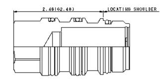
These cavity plugs can be used for both four-port and six-port cavities. When used in four-port cavities (T-21A, T-22A, T-23A and T-24A), ports 1 and 2 remain connected and ports 3 and 4 are blocked. When used in six-port cavities (T-61A, T-62A, T-63A and T-64A), ports 1, 2, 3 and 4 remain connected and ports 5 and 6 are blocked.
