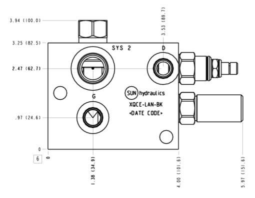
This valve assembly is meant to charge an accumulator using a fixed displacement pump. When the pressure reaches the set point of the valve, the pump is unloaded. When the pressure drops to the value determined by the fixed percentage of the pilot valve, the pump is brought back on line to recharge the accumulator. The ventable relief serves a dual purpose as a main stage to unload the pump and as a system over-pressure relief.
