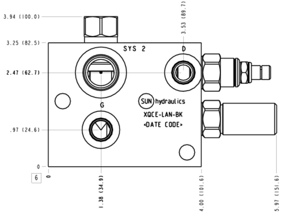
This valve assembly is meant to charge an accumulator using a fixed displacement pump. When the pressure reaches the set point of the valve, the pump is unloaded. When the pressure drops to the value determined by the fixed percentage of the pilot valve, the pump is brought back on line to recharge the accumulator. The ventable relief serves a dual purpose as a main stage to unload the pump and as a system over-pressure relief.
