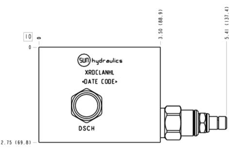
This valve assembly provides a flushing circuit for hydrostatic transmissions. The hot oil flushing circuit allows a discharge of oil from the low pressure side of the loop. The charge pump replaces the hot, dirty oil with cool, filtered oil. The hot oil discharge is often passed through the cases of the pump and the motor, flushing hot, dirty oil from them as well.
