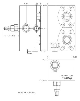
This valve assembly provides a flushing circuit for hydrostatic transmissions. The hot oil flushing circuit allows a discharge of oil from the low pressure side of the loop. The charge pump replaces the hot, dirty oil with cool, filtered oil. The hot oil discharge is often passed through the cases of the pump and the motor, flushing hot, dirty oil from them as well.
