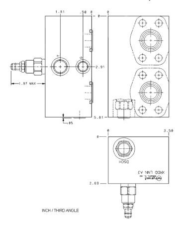
This valve assembly provides a flushing circuit for hydrostatic transmissions. The hot oil flushing circuit allows a discharge of oil from the low pressure side of the loop. The charge pump replaces the hot, dirty oil with cool, filtered oil. The hot oil discharge is often passed through the cases of the pump and the motor, flushing hot, dirty oil from them as well.
