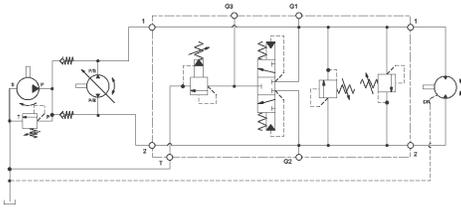
This valve assembly provides high pressure cross-port relief protection and a flushing circuit for hydrostatic transmissions. The hot oil flushing circuit allows a discharge of oil from the low pressure side of the loop. The charge pump replaces the hot, dirty oil with cool, filtered oil. The hot oil discharge is often passed through the cases of the pump and the motor, flushing hot, dirty oil from them as well.
