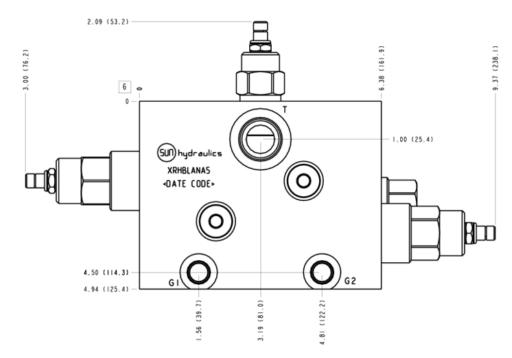
This valve assembly provides high pressure cross-port relief protection and a flushing circuit for hydrostatic transmissions. The hot oil flushing circuit allows a discharge of oil from the low pressure side of the loop. The charge pump replaces the hot, dirty oil with cool, filtered oil. The hot oil discharge is often passed through the cases of the pump and the motor, flushing hot, dirty oil from them as well.
