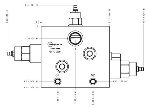
This valve assembly provides high pressure cross-port relief protection and a flushing circuit for hydrostatic transmissions. The hot oil flushing circuit allows a discharge of oil from the low pressure side of the loop. The charge pump replaces the hot, dirty oil with cool, filtered oil. The hot oil discharge is often passed through the cases of the pump and the motor, flushing hot, dirty oil from them as well.
