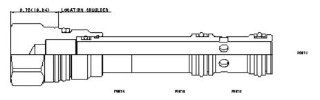
This cavity plug is open from port 1 to port 2, and separately from port 3 to port 4.
