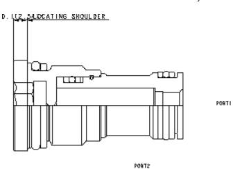
This cavity plug mounts flush with the cavity and blocks all ports.
