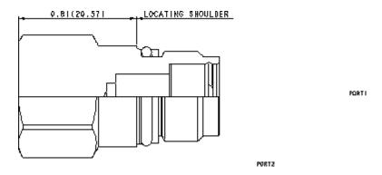
This cavity plug allows all ports to remain open.
