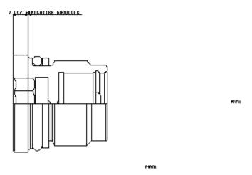
This cavity plug mounts flush with the cavity and allows all ports to remain open.
