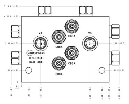
This assembly is a combination of the cushion lock circuit and flow dividers. It provides flow division to two actuators in both directions. It provides overrunning load control in both directions. It provides cross-port relief protection. It provides thermal relief protection. It supplies make-up oil. It flushes hot and dirty oil out of the actuators.
