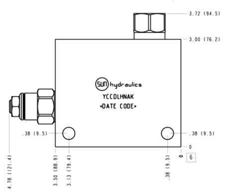
This valve assembly provides overrunning load-control, load-port relief protection, supplies make-up oil, and flushes hot dirty oil out of the actuator. All oil coming out of the actuator returns to tank through port T.
